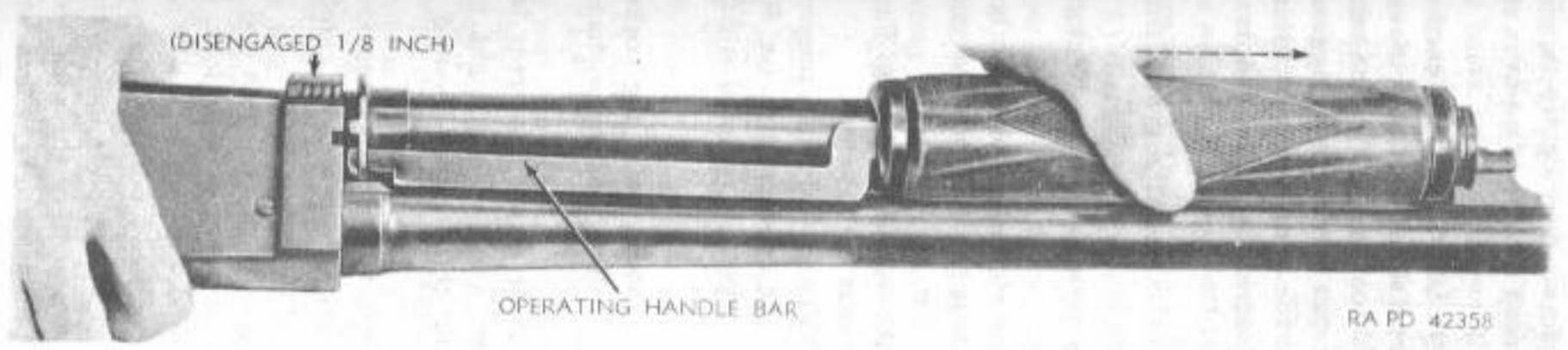
Figure 49—Disengaging Operating Handle Bar—Stevens Shotgun M620
